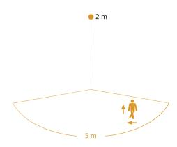
Possible mounting height: 1,80 m - 2,50 m Orange: radial and tangential
